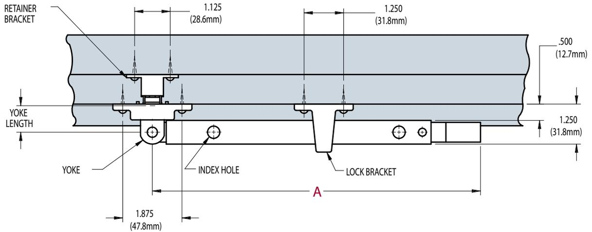
YOKE LENGTH = PIVOT RIVET TO YOKE RIVET
