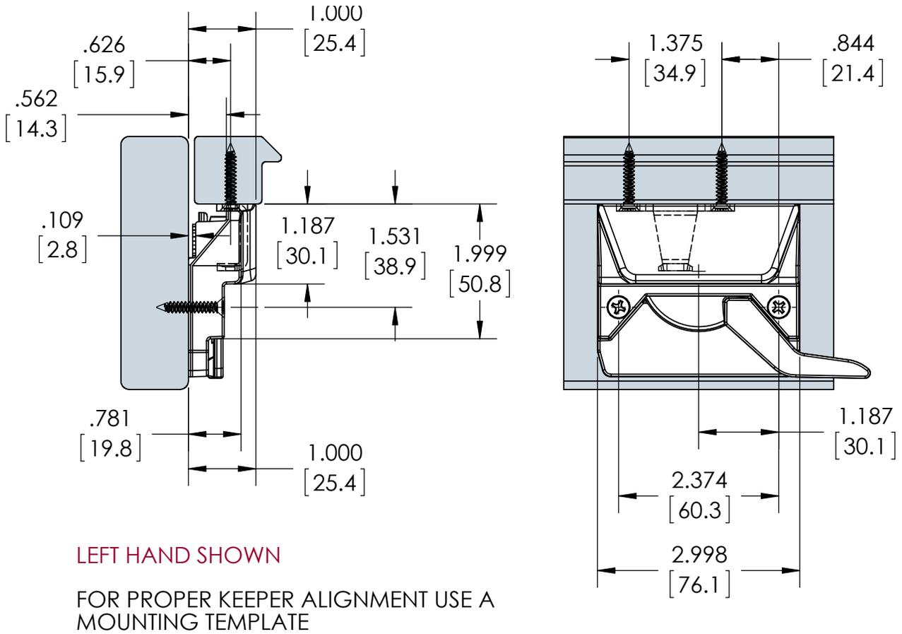
FIG. 2 16.27 AND 16.30 CASEMENT SASH LOCK
