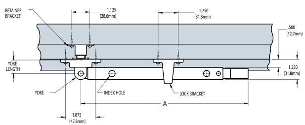
YOKE LENGTH = PIVOT RIVET TO YOKE RIVET
