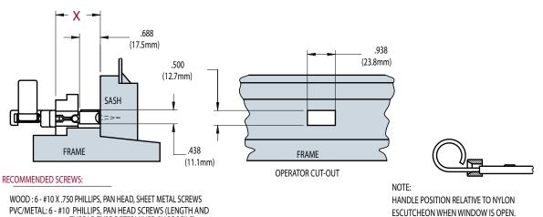
PVC/METAL: 6 - #10 PHILLIPS, PAN HEAD SCREWS (LENGTH AND THREAD TYPE DETERMINED BY PROFILE)
