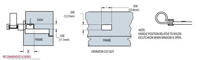
WOOD : 6 - #10 X .750 PHILLIPS, PAN HEAD, SHEET METAL SCREWS PVC/METAL: 6 - #10 PHILLIPS, PAN HEAD SCREWS (LENGTH AND THREAD TYPE DETERMINED BY PROFILE)
