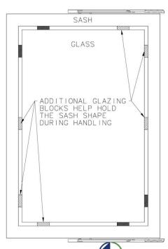
54.812". The difference between the diagonals is 55.000 - 54.812 = .188". The amount of sash sag is roughly 60% of .188" which is .60 x .188 = .113" of sash sag.
